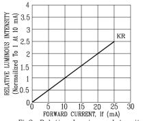
g3. Relative Luminous Intensity vs. DC Forward Current
